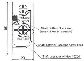
[Checking the alignment of the red slot line on the Shaft Setting/Resetting screw head]
