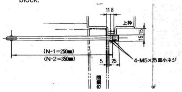
Fit the door selector underneath to the top frame. There should be a space of 5mm between fixing block and the door leaf.
