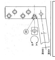
The angle of the arm can be adjusted with the screw in front of the fixing block. The arm should be set in such position that the first door to close can pass.
